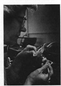
EVEN TRANSFORMERS occasionally require the use of a magnifying glass. Marie K. Carlson is placing three windings of finer-than-hair copper wire around the tiny cores. The Transformer Shop has its own "clean room" for use when dustfree environment is required in working with minute assemblies.
